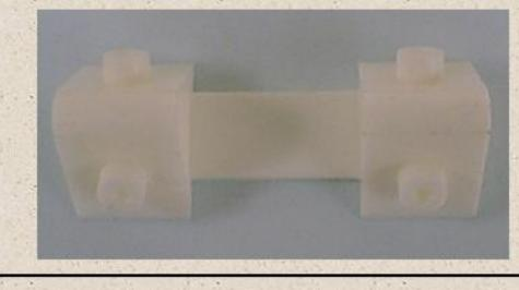
**Example of Objects Produced Using Multi-Stage Molding**
