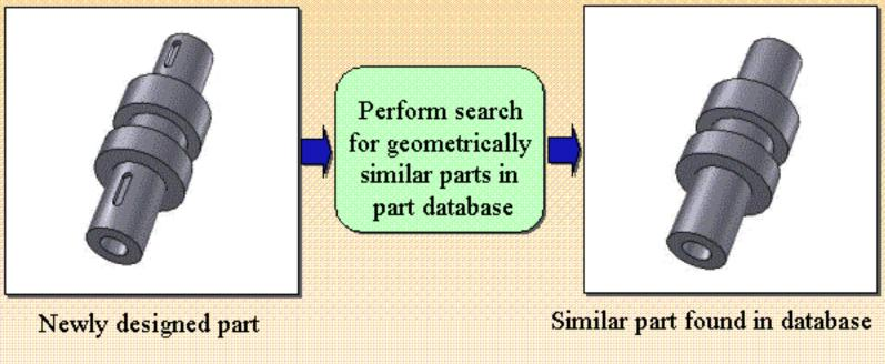
New part can be produced by cutting two slots in the existing part
