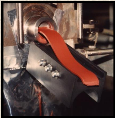
Energetic Material Continuously Extruding from Die of TSE
