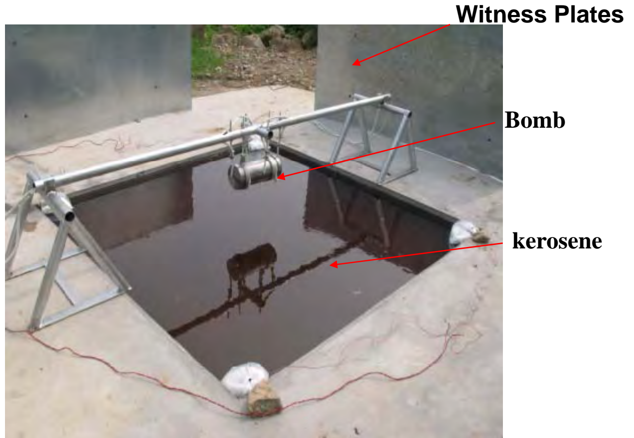
Photograph of Fire Cook-off test
