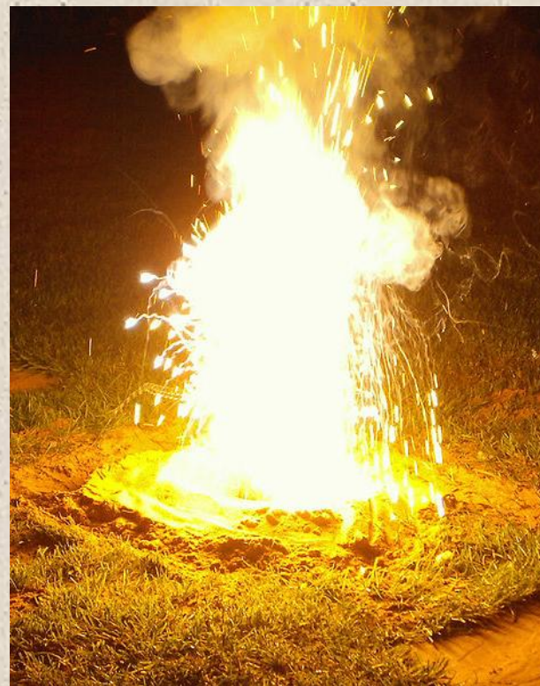
Al/Fe 2 O 3 Thermite Reaction
