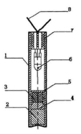
The structure of electric detonator with NHN
