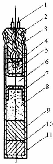
Drawing: The simple flying plate electric detonator without primary explosive
