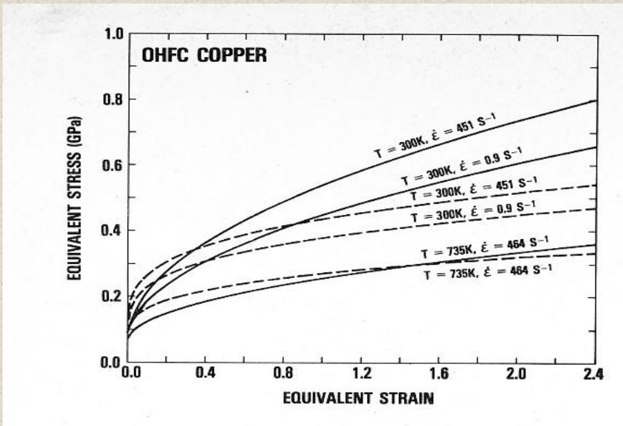
$B_0 = 890\text{ MPa}$ ,  $\alpha_0 = 0.0028\text{ K}^{-1}$ ,  $\alpha_1 = 0.000115\text{ K}^{-1}$ ,  $(\varepsilon/\varepsilon_r) < 1.0$ ,  $k_\varepsilon = 5\text{ MPa}\cdot\text{mm}^{1/2}$ ,  $\sigma_G + k_\varepsilon l^{-1/2} = 65\text{ MPa}$
