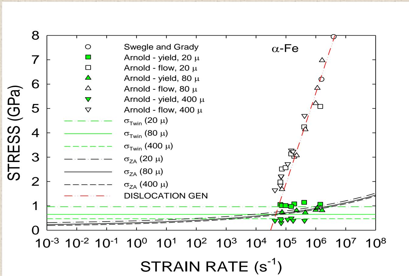
Plastic front propagation by nanoscale twinning
