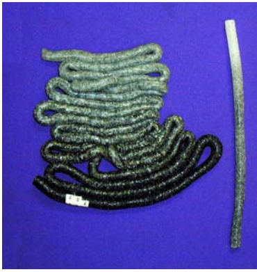
Figure 4. Graded Composites manufactured using the TSE process
