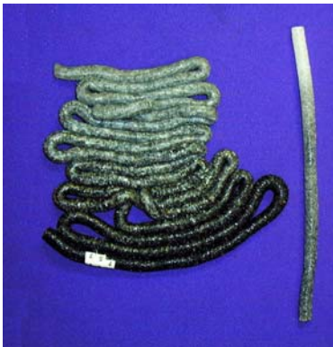
Figure 5. Graded polymer composites manufactured using the TSE process
