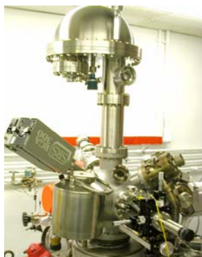
Figure 2. UHV apparatus for in-situ surface analysis of vapor deposited nitramines.
