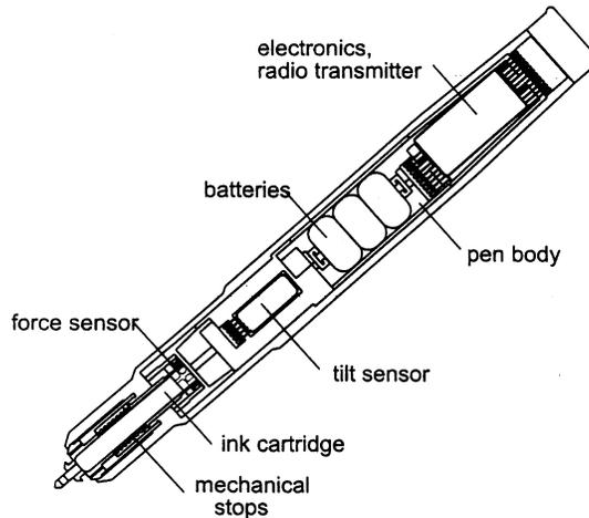
Fig. 1. SmartPen system [1] (Courtesy of IEEE).
