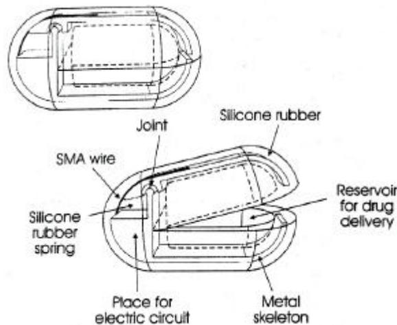
Fig. 2. Solid drug delivery device [1] (Courtesy of IEEE).
