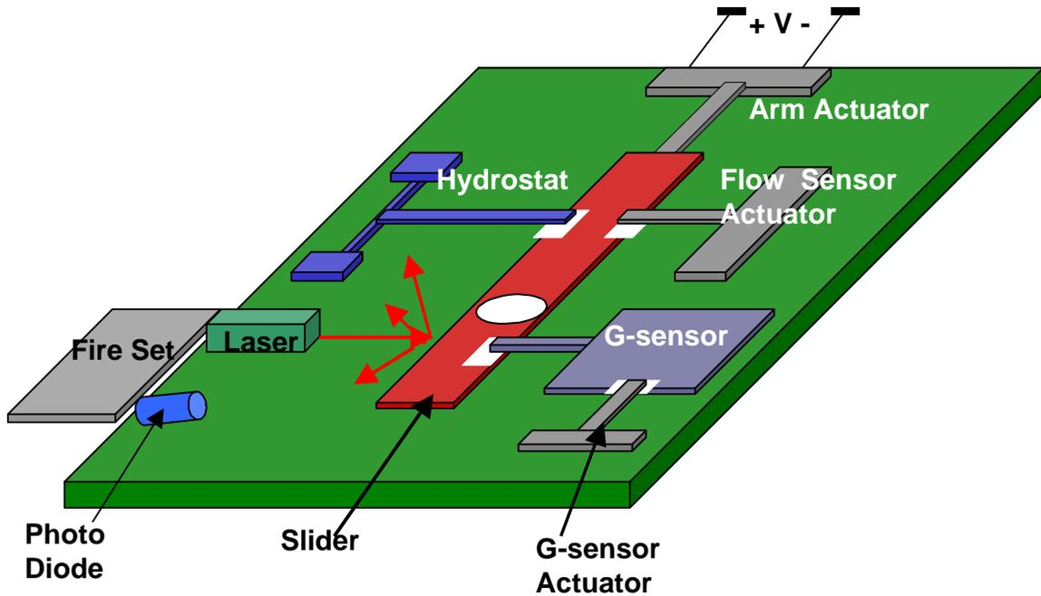
Fig. 4. Key components of the S&A fuze systems.
