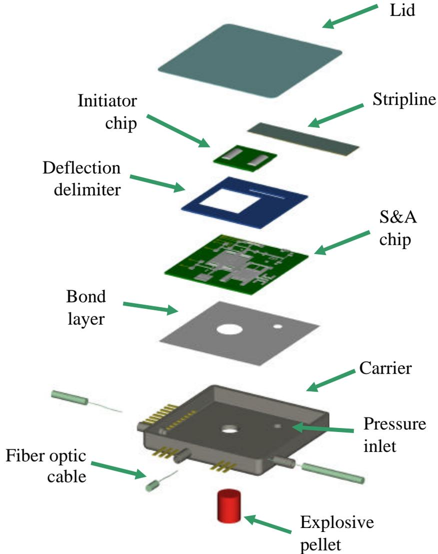
Fig. 5 Carrier-level package.
