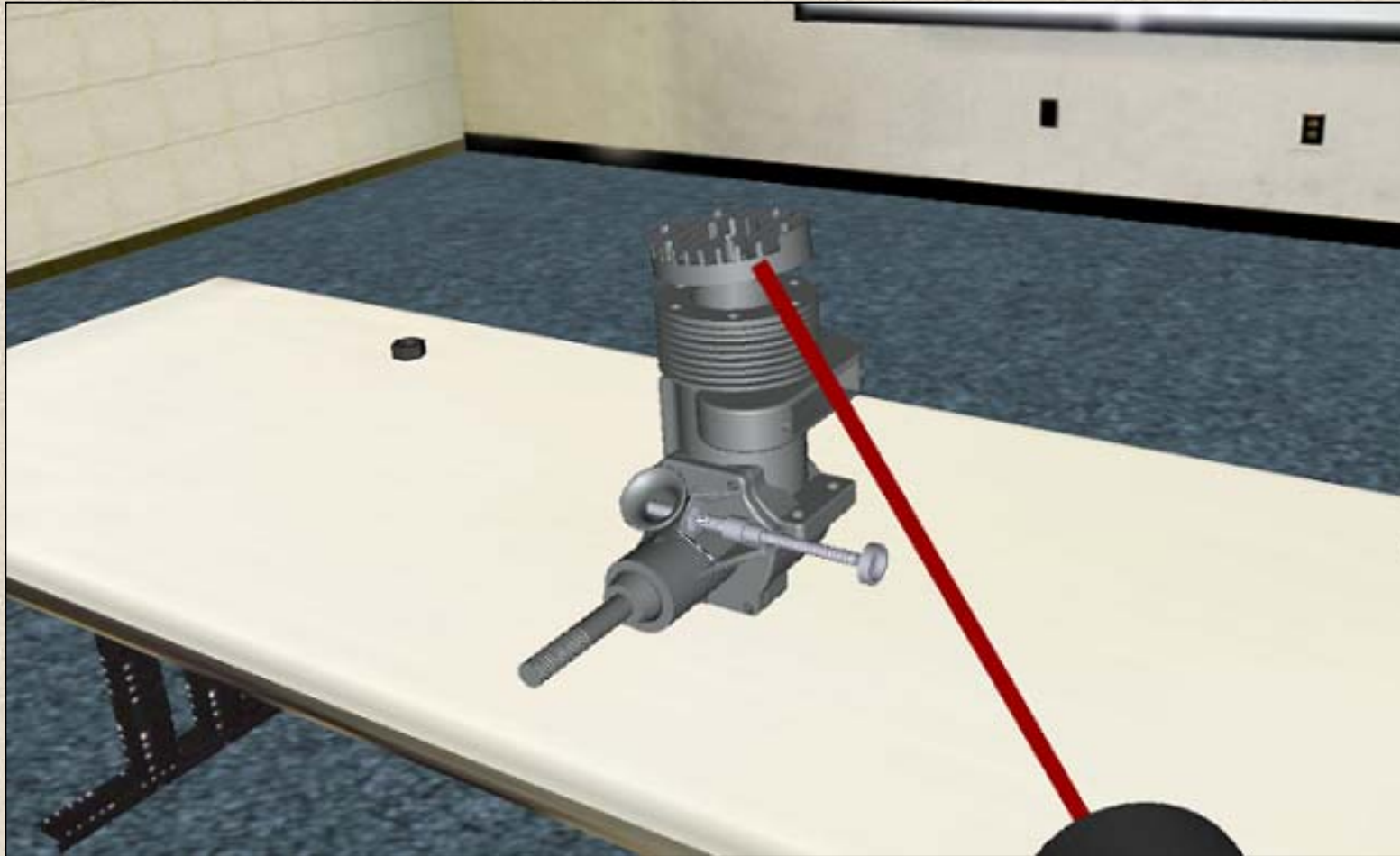
Figure 5: Virtual demonstration of attachment of engine cover to top of engine case
