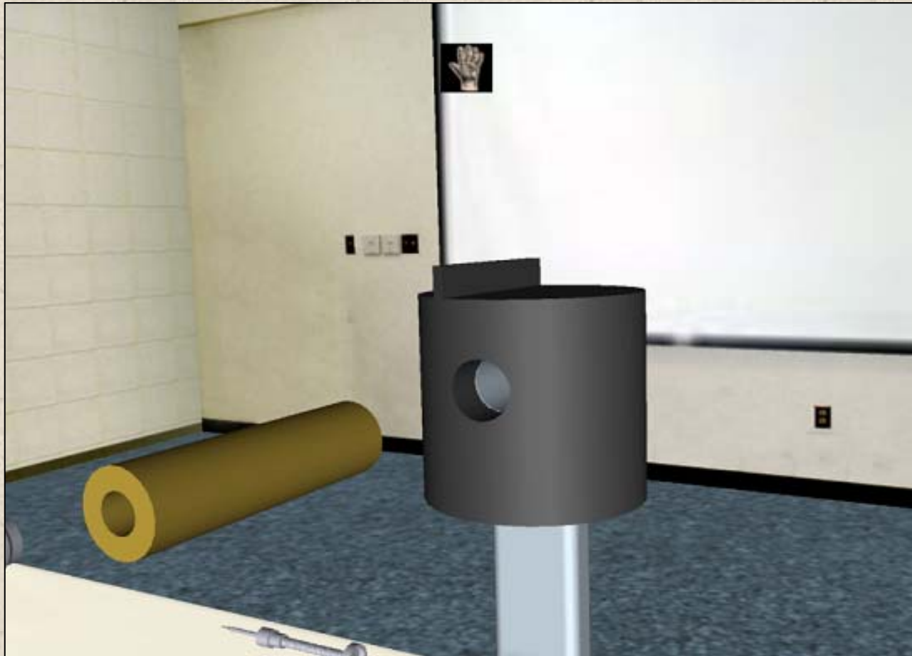
Figure 8: An example of subtype B4 symmetry where the pin can be inserted from two different positions (either side of the piston hole). For each position either the alternate or the primary orientation around the secondary axis may be used.
