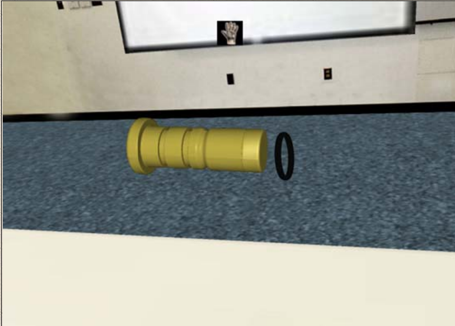
Figure 14: Rubber o-ring must be rolled on top of the rightmost rectangular groove.
