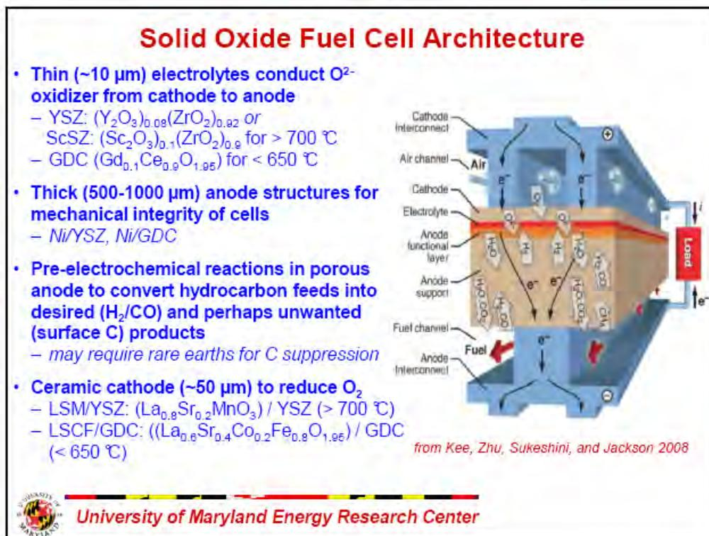
**Figure 3 - solid oxide fuel cell architecture**
