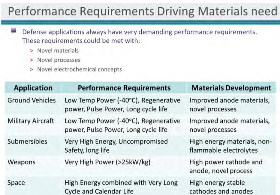
**Figure 10 – Saft Groupe performance requirements driving specialty batteries’ material design**
