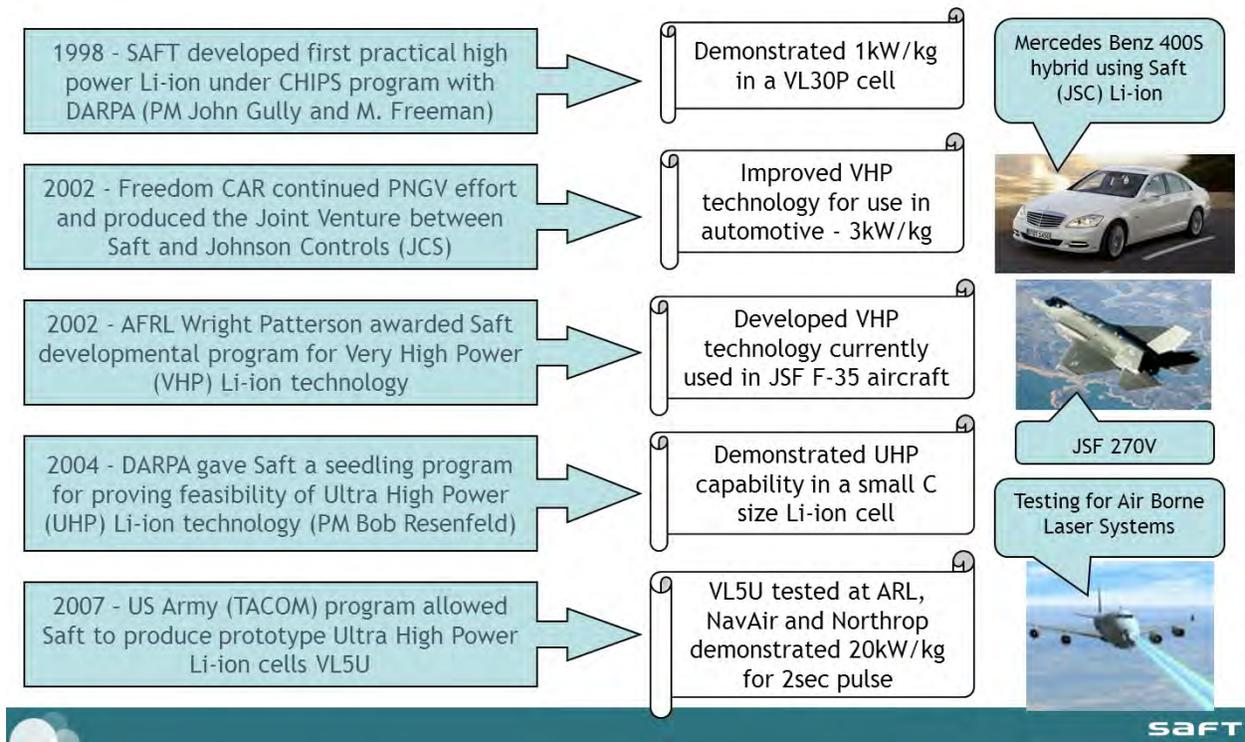
Figure 12 - Development of a practical high power Lithium Ion battery for DOD applications at SAFT
