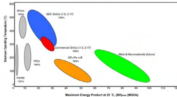
**In the last 100 years, the strength of the magnets [(BH)<sub>max</sub> and H<sub>c</sub>] increased dramatically (by a factor of 100)
