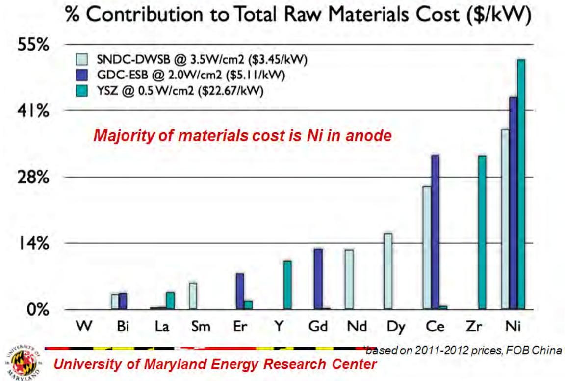
**Figure 6 – SOFC relative material costs**
