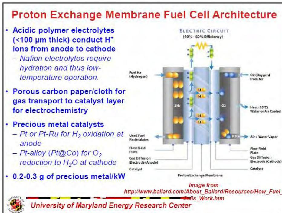
Figure 2 - Proton exchange membrane fuel cell architecture
