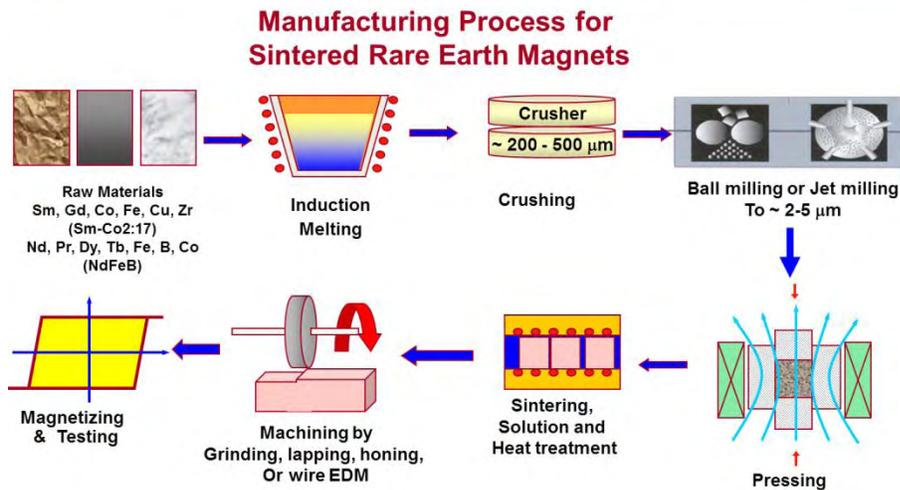
**Figure 13 – Manufacturing process for sintered rare earth magnets**
