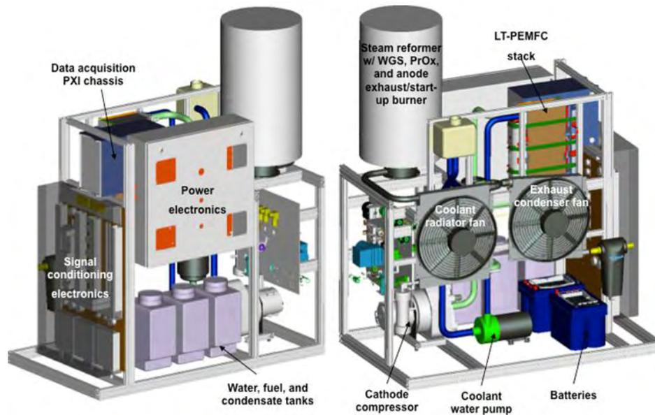
**Figure 4 – Ballard/UMD system for 1-5 kWe prototype PEM fuel cell system for hydrocarbon fuels**
